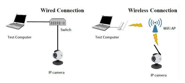
Figure 11 Test Setup
