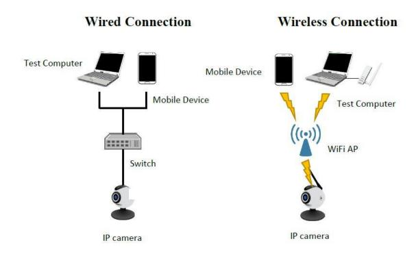
Figure 19 Test Setup
