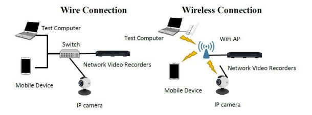
Figure 26 Test Setup
