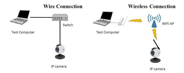
Figure 4 Test Setup
