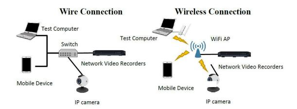
Figure 24 Test Setup
