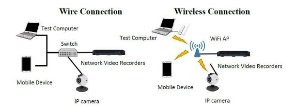
Figure 21 Test Setup
