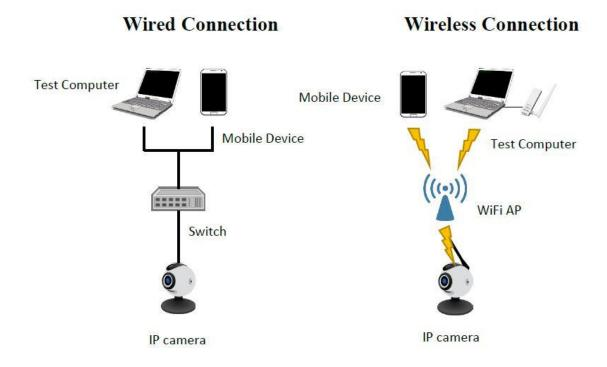
Figure 14 Test Setup
