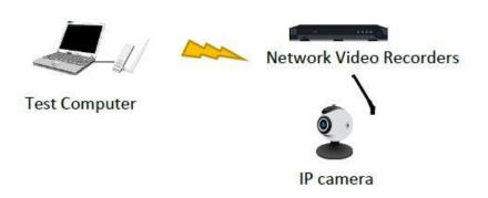
Figure 28 Test Setup
